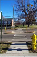
Pedestrian-activated traffic signals at pedestrian crossings allow a pedestrian to activate a traffic signal in mid-block locations. National standards now include guidelines that help identify locations where pedestrian volumes warrant such signal installations.
